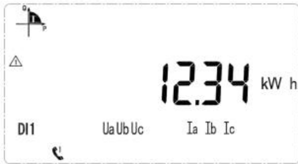
Current forward active energy 12.34kWh
