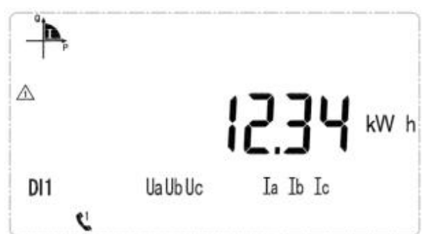
Current forward active energy 12.34kWh
